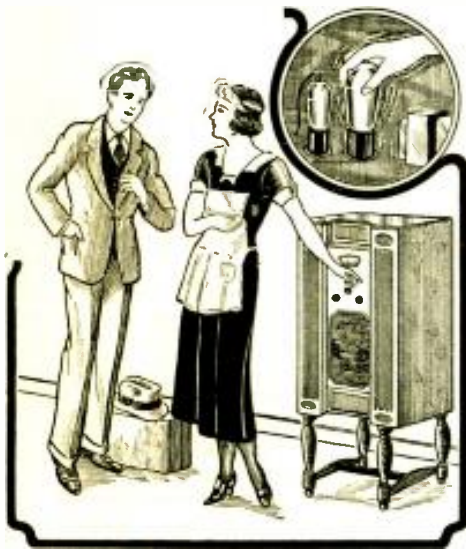
"We make it come back by wiggling the big tubes in their sockets."
