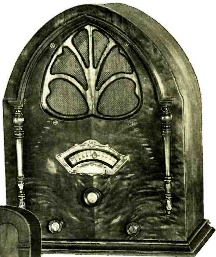
4 Tube Short Wave Converter. Uses 1-27; 1-21; 1-51; 1-80. Triple Switching Arrangement. No plug-in coils. Full-vision dial with travelling light. Special two-toned Walnut cabinet. Adapter connected to any receiver makes it a superheterodyne on short waves. Power supply is self-contained unit. Used on AC or battery operated receivers. Smooth tuning by means of high ratio tuning dial. Height 11½", Width 13½". Depth 9½". AC Model, $14.25 less tubes. COMPLETE WITH ARCTURUS TUBES $16.25.
